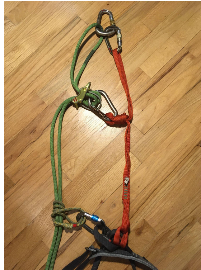
Anchor and extension with nylon sling with overhand on a bight knot
