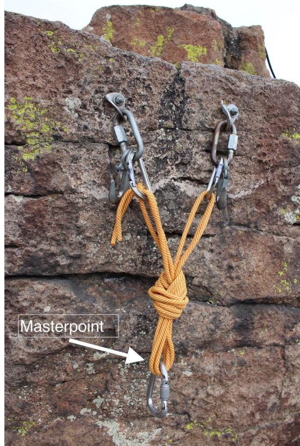
2 point cordelette anchor, bolts
